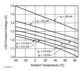
Figure 1. LED Voltage vs. Temperature
