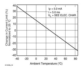
Figure 4. Current Limit vs. Temperature
