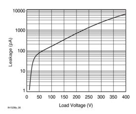
Figure 8. Leakage Current vs. Applied Voltage
