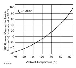
Figure 2. LED Current for Switch Turn-on vs. Temperature
