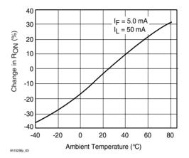
Figure 3. ON-Resistance vs. Temperature
