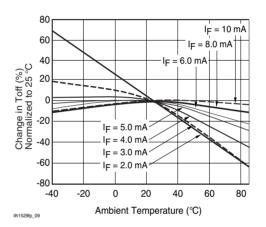
Figure 9. Turn-off Time vs. Temperature
