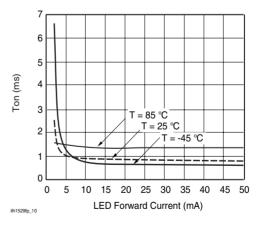
Figure 10. Turn-on Time vs. LED Current
