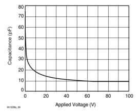
Figure 6. Switch Capacitance vs. Applied Voltage
