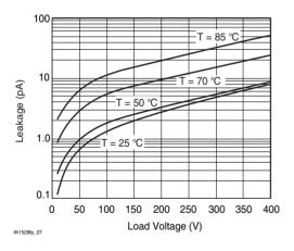
Figure 7. Leakage Current vs. Applied Voltage
