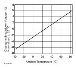
Figure 5. Switch Breakdown Voltage vs. Temperature
